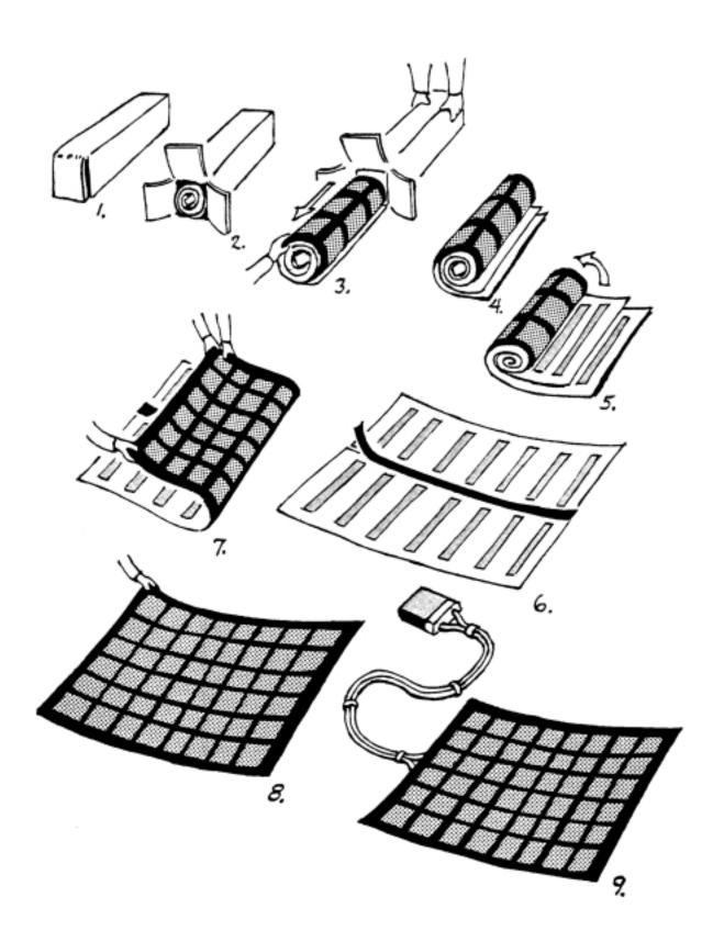
Remove the control module from its bag and plug the cables from the Electric Maze™ grid into the control module. The cables' end connectors and the control module's connectors are color coded with red and blue dots. Secure the cable connectors with their knurled screws to ensure proper electrical contact.
