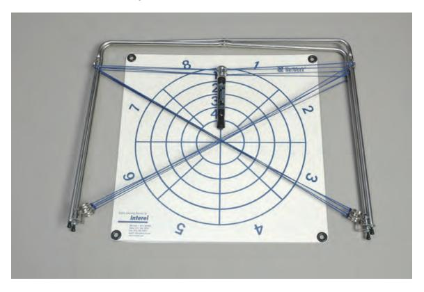
Open the hinged frame to a cross shape and place, rubber feet down on a flat surface, over the desired target
